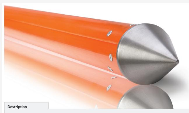
QD (Quick Drive) Casing has all the advantages of EC (Easy Connect) Casing, combined with a mild steel nose cone for driving into preformed window sampling holes, and may also be used for shallow installations into soft soils.
